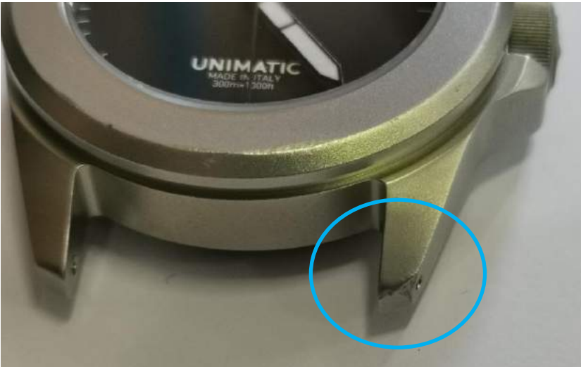
Figure 5 – Example of dents caused by the impacts
