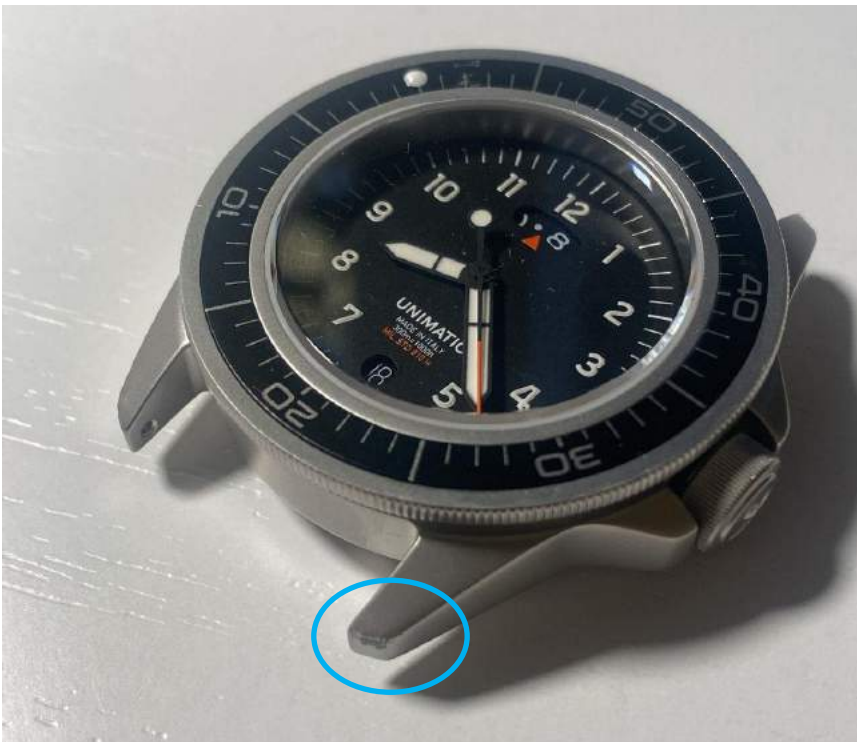
Figure 4 – Example of dents caused by the impacts
