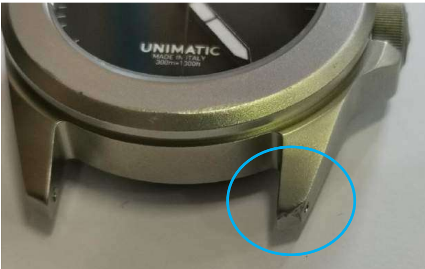
Figure 5 – Example of dents caused by the impacts
